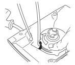
Undo the screw in the centre of the pulley and remove the pulley. Insert and fasten a new starter cord to the pulley. Wind approx. 3 turns of the starter cord onto the pulley. Connect the pulley to the recoil spring so that the end of the spring engages in the pulley. Fit the screw in the center of the pulley. Insert the starter cord through the hole in the starter housing and the starter handle. Make a secure knot in the end of the starter cord.
