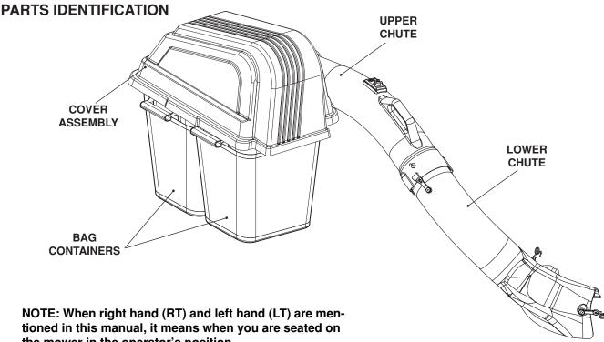
the mower in the operator's position.
