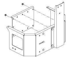
Secure collection guard assembly to the mower frame at the side where rear guard was removed. Use two on <sup>3</sup>/<sub>8</sub>-16 x <sup>3</sup>/<sub>4</sub> round head bolts and nuts on each side.
