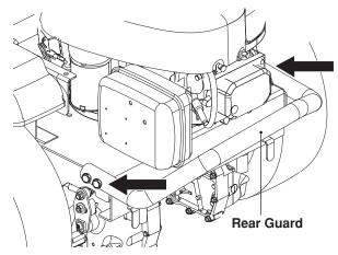
Using round head <sup>5</sup>/<sub>16</sub>-18 x <sup>3</sup>/<sub>4</sub> bolts and nuts, assemble the hanger bracket to the rear guard sections and the rear support plate. Use the illustrations for orientation of hardware according to mower size. For the 30" mower, the rear guard sections will fit together. For the 42" mower, the sections will be have a gap of approximately 2".
