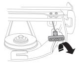
6 Loosen on the cutting height stay and place in the holder.
