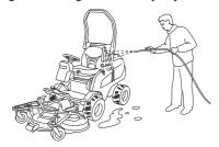
Oily dirt can be removed using a cold degreasing agent. Spray on a thin layer.
