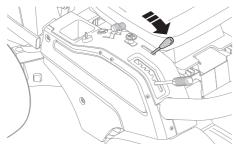
When cutting the lever should be set directly to the floating position (3).
