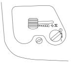
2 When the Rider is at a standstill, press down the parking brake and push in the locking button.
