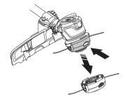
Pull out the line chute assembly.
