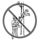
5 You must have a steady stance in order to have full control over the chain saw. Never work standing on a ladder, in a tree or where you do not have firm ground to stand on.
