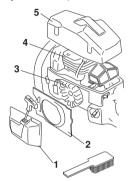
Clean the cooling system with a brush once a week, more often in demanding conditions. A dirty or blocked cooling system results in the machine overheating which causes damage to the piston and cylinder.
