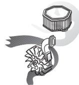
**IMPORTANT!** In order to maintain operation of the centrifugal cleaning system it must be regularly maintained. Clean the air intake to the starter, the fins on the flywheel, the space around the flywheel, inlet pipe and carburetor compartment.
