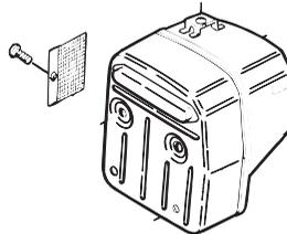
Some mufflers are equipped with a special spark arrester screen. If your machine has this type of muffler, you should clean the screen at least once a week. This is best done with a wire brush. A blocked screen will cause the engine to overheat and may lead to serious damage.
