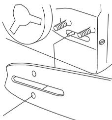
Tension the chain by turning the chain tensioning screw clockwise using the combination spanner.
