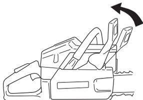
Remove the bar nuts and remove the clutch cover (chain brake). Take off the transportation guard (A).
