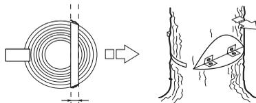
All control over the felling direction is lost if the felling hinge is too narrow or non-existent, or if the directional cuts and felling cut are badly placed.
