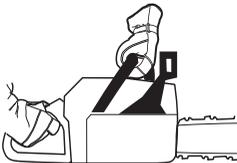
Apply full throttle and activate the chain brake by tilting your left wrist forward onto the front hand guard. Do not
