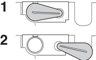
**CAUTION!** When the plug is fitted in the air nozzle for "Air injection" the air filter must be cleaned at least once every day.
