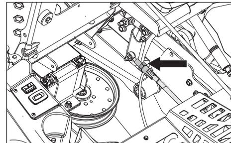
4. Remove and retain the pin from the front coupler.
