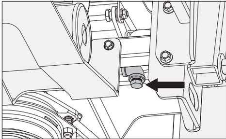
5. Let the oil to fully drain from the engine.
