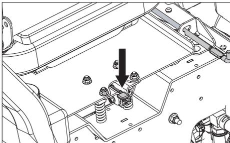
The seat can be rotated forward to access the mower battery and hydro gears. Push down on the latch lever to release the seat. Raise the seat until the rod engages.
