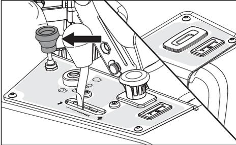
The choke control is used for cold starts to provide the engine with a richer fuel mixture. For cold starts, pull the control up.
