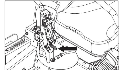
3. To change the park brake action, tighten the pivot bolt until the desired braking feel is correct.
