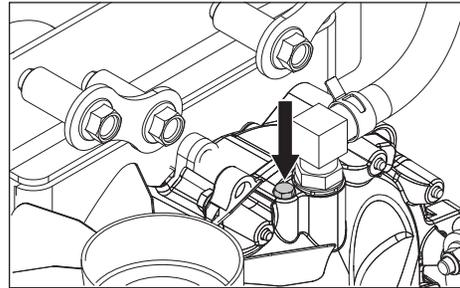
8. Fill with 20W50 motor oil until the oil appears at the bottom of each transaxles' top port, approximately 2 quarts (1.89 liters) per transaxle, 4 quarts (3.78 liters) total.
