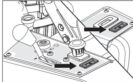
Fuel gauges for each fuel tank are located the right and left control panels.
