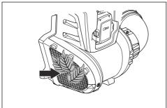
Stop the product and remove unwanted material if it is necessary.
