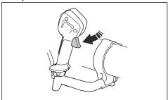
Push the Cruise control button to set the selected airflow. The LED comes on.
