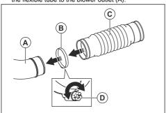
2. Make sure to put the clamp screw (D) as the illustration shows. Tighten the screw.
