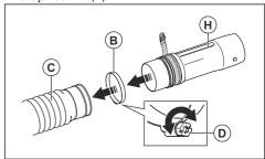
Make sure to put the clamp screw (D) as the illustration shows. Tighten the screw.
