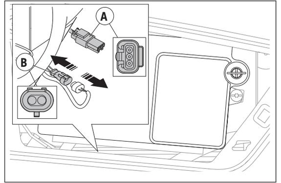
6. Connect the CAN bus and Husqbus connectors to the Husqvarna Service Interface Box
