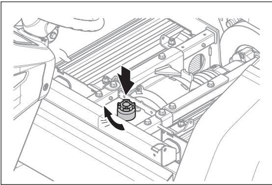
4. Remove the service lid by unscrewing the 2 screws
