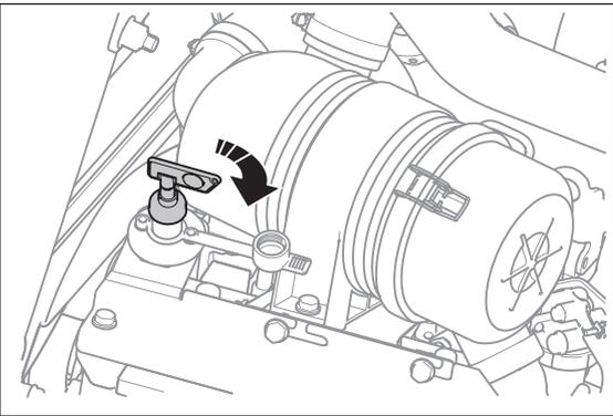
3. Make sure that 48V servicing plug are installed
