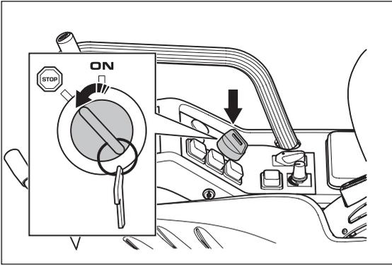
2. Push down and turn the main switch to the ON position
