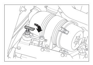
3. Make sure that 48V servicing plug are installed
