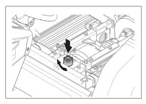
4. Remove the cover of the steering column
