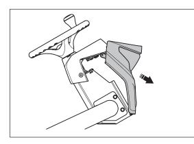
5. Move the rubber seal to side and connect the USB cable to the USB port on the Display
