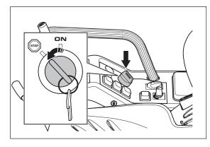
2. Push down and turn the main switch to the **ON** position
