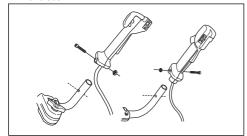
Align the screw hole in the throttle handle with the hole in the handlebar.
