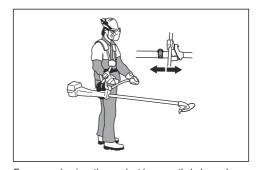
For grass clearing, the product is correctly balanced when the blade is at cutting height near the ground.
