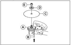
Make sure that the drive disc and support flange engages correctly in the center hole of the grass blade.
