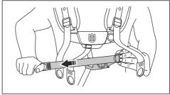
12. Adjust the height of the suspension point, see *Product overview on page 2.* For forestry clearing, the correct height of the suspension is approximately 10 cm below your hip bone.
