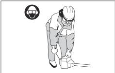
Pull the starter rope handle slowly until you feel some resistance, then pull the starter rope handle with force.
