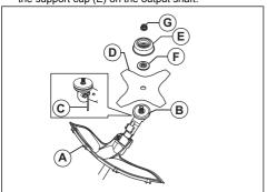
Make sure that the drive disc and support flange engages correctly in the centre hole of the grass blade.
