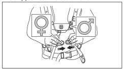
9. Tighten the elastic strap (B) to move more load from the shoulder strap to the hip strap.
