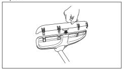
Release the locking hooks with the spark plug wrench to remove the guard extension.
