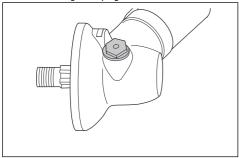
Look into the grease plug hole and turn the drive shaft. The grease level (A) must be in level with the top of the gear cogs (B).
