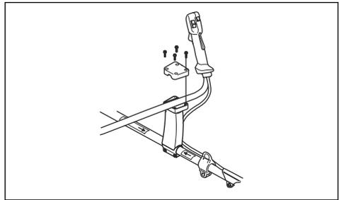
2. Make sure that the holes for the screws align.
