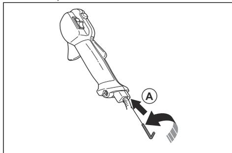
4. If the start throttle speed is too high, turn the adjuster screw (A) counterclockwise until the cutting attachment stops. Turn the adjuster screw (A) clockwise 1/2 turn more.
