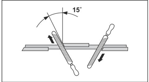
**Note:** Sharpen the edges of the teeth with a flat file if the blade is heavily worn. Continue to sharpen with a round file.
