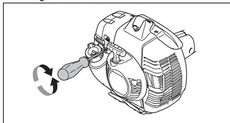
2. Turn the idle adjustment screw counterclockwise until the cutting attachment stops.
