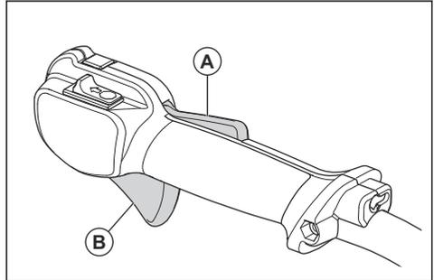
2. Push down the throttle trigger lockout and make sure that it goes back to its initial position when you release it.
