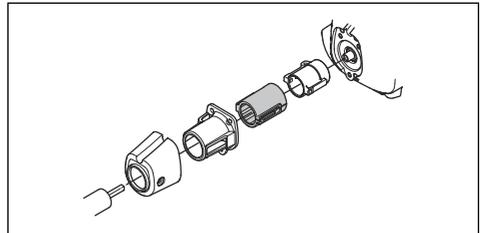
3. Make sure that the vibration damping units are correctly attached.
