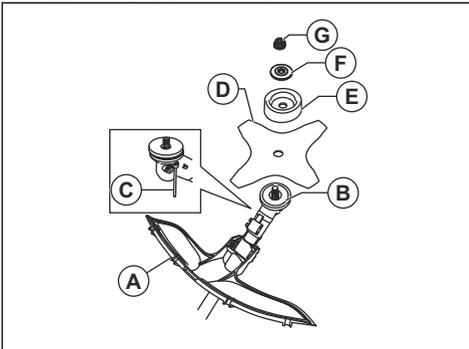
6. Make sure that the drive disc and support flange engages correctly in the centre hole of the grass blade.
