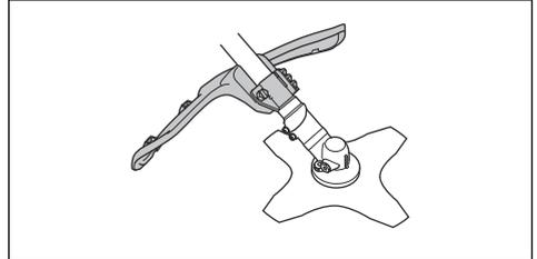
2. Replace the cutting attachment guard if it is damaged.
