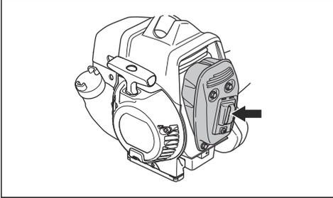
3. If your product has a special spark arrester screen, clean the spark arrester screen weekly.
