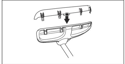
2. Put the guard extension into position on the cutting attachment guard with the 4 locking hooks.
