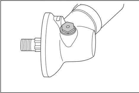
4. Look into the grease plug hole and turn the drive shaft. The grease level (A) must be in level with the top of the gear cogs (B).
