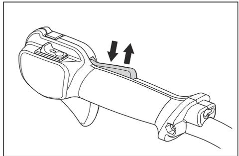
3. Make sure that the throttle trigger is locked at the idle position when the throttle trigger lockout is released.
