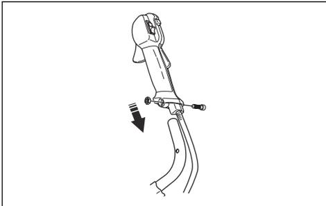
2. Move the throttle handle to the right side of the handlebar.
