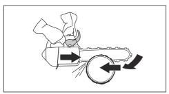
To cut on the push stroke is when you cut with the top of the guide bar. The saw chain pushes the product in the direction of the operator.
