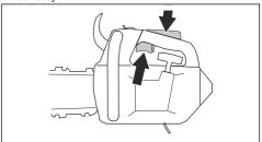
Push down the throttle trigger lockout and make sure that it goes back to its initial position when you release it.
