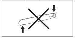
Make sure that the bar tip sprocket turns freely and that the lubricating hole in the bar tip sprocket is not blocked. Clean and lubricate if it is necessary.
