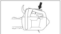
Make sure that the throttle trigger is locked at the idle position when the throttle trigger lockout is released.
