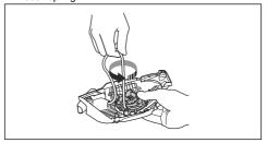
5. Remove the bolt in the center of the pulley and remove the pulley.
