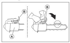
Pull the front hand guard rearward to disengage the chain brake
