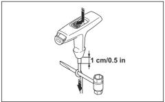
**Note:** If the starter rope is broken in the starter rope handle, push the starter handle cover down. Use the combination wrench to remove the starter handle cover.
