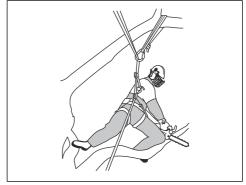
Use a foot loop to keep a safe work position.
