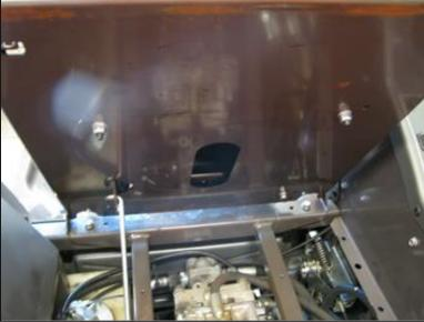
Dismount the original seat by loosening the four nuts underneath the seat mount bracket/plate, also loosen the cable for the safety switch.
