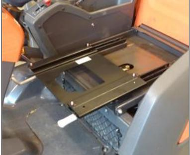
Mount the bottom part of the slide rails for the seat, on top of the square tube, with the Insex bolt M8 \* 45 through the seat mount bracket/plate, and secure with nuts underneath. Then you slide the horizontal isolator t kit on to the mounted slide rails.
