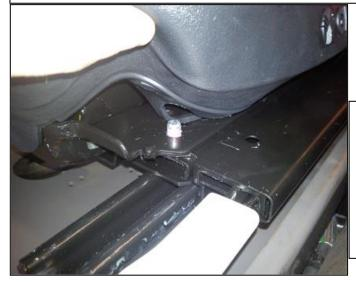
Mount the seat on to the horizontal isolators fixed threaded M8 bolts, the seat should be mounted using the hole in the front of the seats mounting plate. Secure the seat with M8 nuts.
