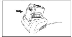
Make sure that the green charging light on the battery charger comes on. That means that the battery is connected correctly to the battery charger.
