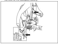
2. Adjust the harness to optimize the work position.
